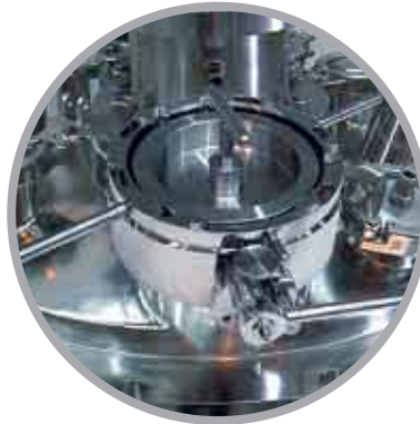
Pressure Rated ChargePoint® with Pressure Rated Plug in place
