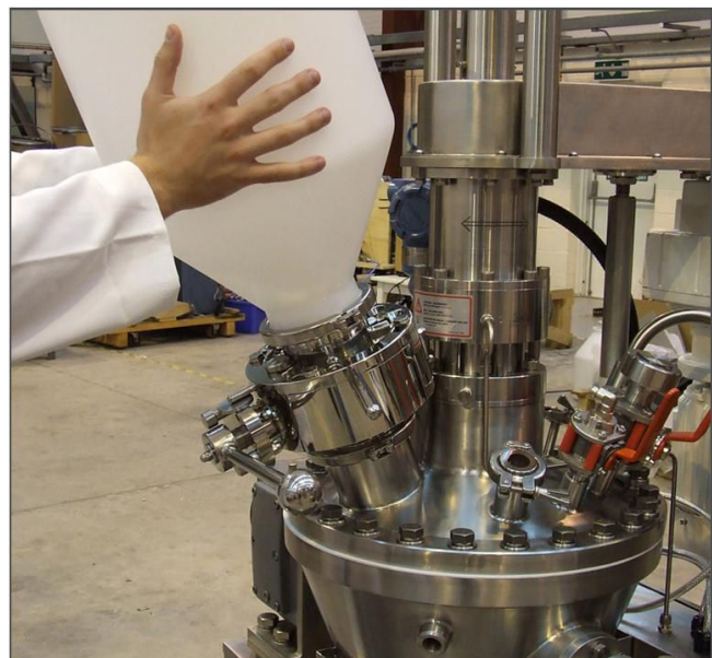
Reactor vessel showing the ChargePoint installed and fitted with a pressure rated sightglass Passive (left) and pressure rated ChargeBottle Passive (right)
