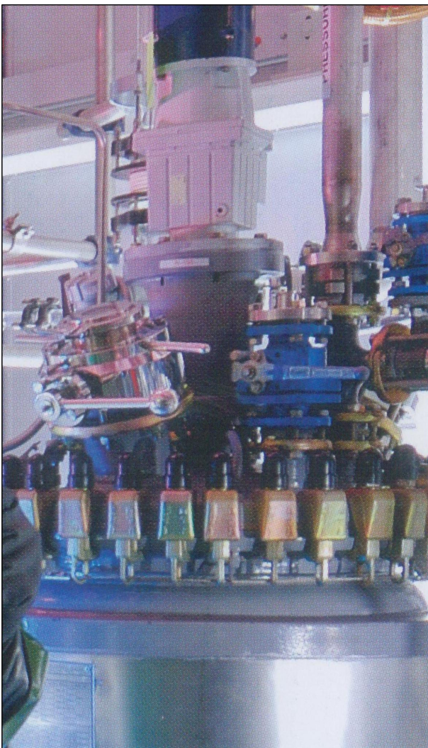
Reactor vessel showing the ChargePoint installed and fitted with a pressure rated sightglass Passive (left) and pressure rated ChargeBottle Passive (right)
