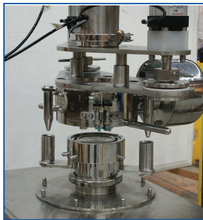
Figure 3: SBV with integrated automated docking system
