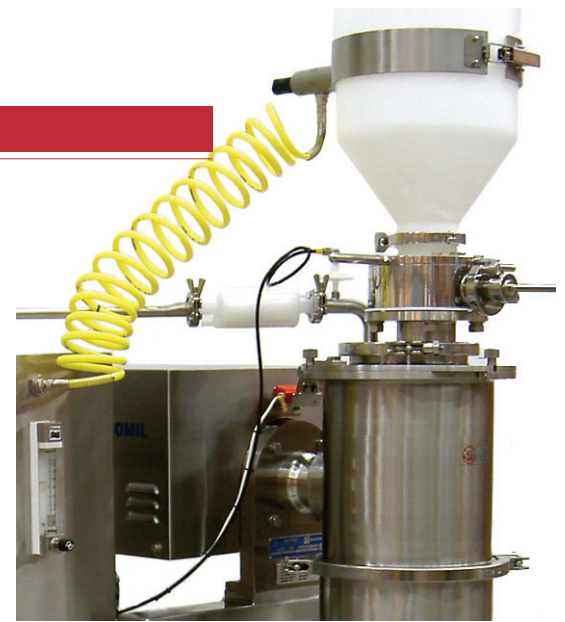
Figure 2: A vibratory collar to aid charging of cohesive product through a SBV to a mill
