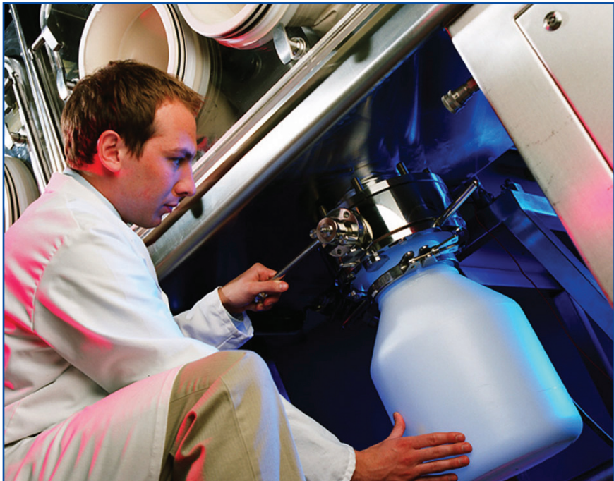
Correct split valve selection can be crucial to containment performance and ease of operation
