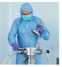
Once mated, the disc can be opened. This allows the product to be securely transferred from transfer container to vessel, eliminating the risk of contamination. Performing this transfer within the grade C space provided considerable cost and production benefits.
